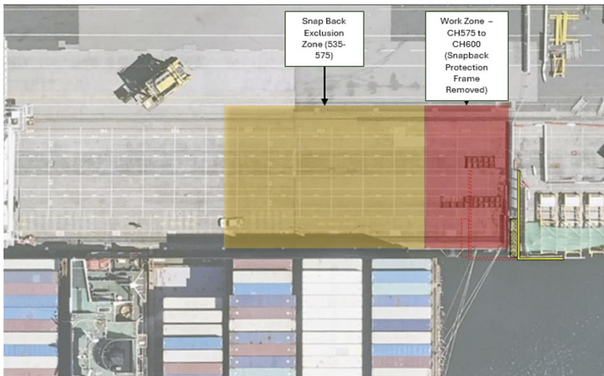
Swanson Dock West Berth 2 – Works Zone Diagram
